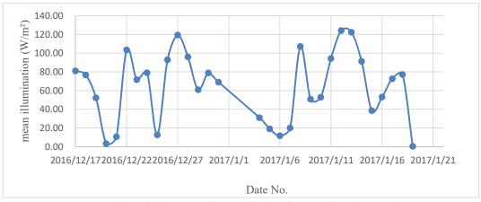
Figure 7. The variation curve of mean illumination outside solar greenhouse
